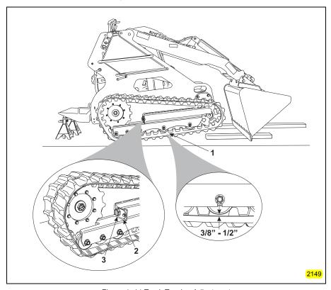
Figure 4-14 Track Tension Adjustment
